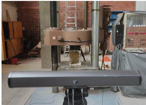
Setup of the OptoTrack system
